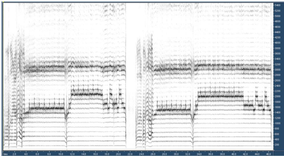
Figure 10. Tuvan *Sygyt* style. The fundamental is a weak E3+ 167 Hz. The melody uses the 8<sup>th</sup> (E6+ 1336 Hz), 9<sup>th</sup> (F#6+ 1503 Hz), 10<sup>th</sup> (G#6+ 1670 Hz) and 12<sup>th</sup> (B6+ 2004 Hz). There is a rhythmic shift between contiguous harmonics each 900 ms. In the 3000-3200 Hz zone, we can see a second resonance region.
