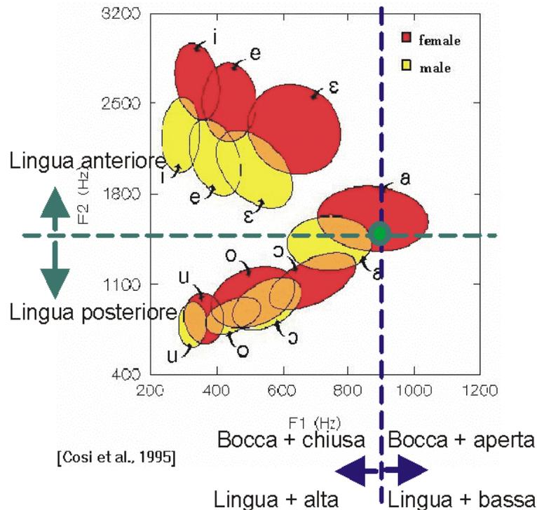
Figure 4. Opening the mouth controls the 1<sup>st</sup> formant position. The movement of the tongue affects the 2<sup>nd</sup> formant and allows the harmonic selection in a large frequency range.
