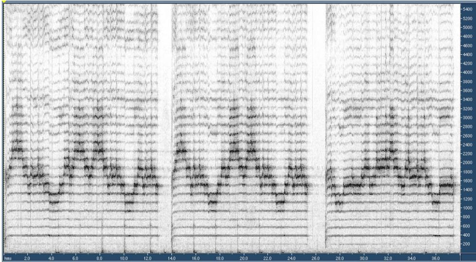
Fig. 6 Tuvan *Khomei Style*. The fundamental is a weak F#3+ 189 Hz. The diphonic harmonics are the 6<sup>th</sup> (C#6+ 1134 Hz), 7<sup>th</sup> (E6 1323 Hz), 8<sup>th</sup> (F#6+ 1512 Hz), 9<sup>th</sup> (G#6+ 1701 Hz), 10<sup>th</sup> (A#6+ 1890 Hz) and 12<sup>th</sup> (C#7+ 2268 Hz).
