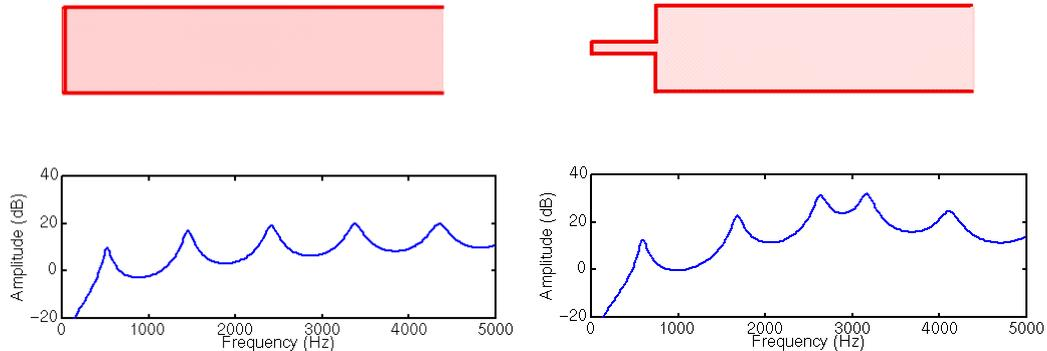
Figure 3. Resonance envelope for an uniform vocal tract (left). A constriction on the pharynx moves the formants so that the intensity of partials in the 2500-3500 Hz region increases (right).
