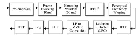
Fig. 1. PMVDR feature extraction process.
