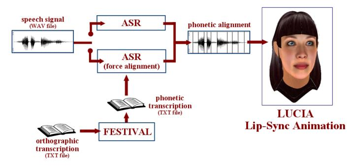
Figure 3: LW2A's block diagram. In the upper branch, the application accepts in input only the speech signal (WAV file) while in the lower branch a speech signal (WAV file) and its corresponding orthographic transcription (TXT file) are both needed.
