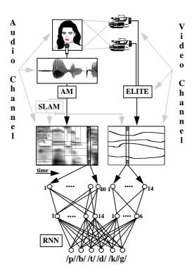
Figure 1. Structure of the bimodal recognition system.
