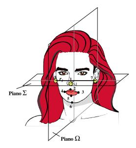
Figure 2. Position of the reflecting markers and of the reference plane. Identification numbers are indicated next to their corresponding markers. Marker dimension in the figure does not correspond to the real dimension (2mm) but is exaggerated for visualization purpose.
