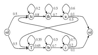
Figure 2. HMM state sequence for a two-word vocabulary.
