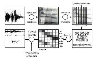
**Figure 1**. Graphical overview of the recognition process, illustrating recognition of the word "two".
