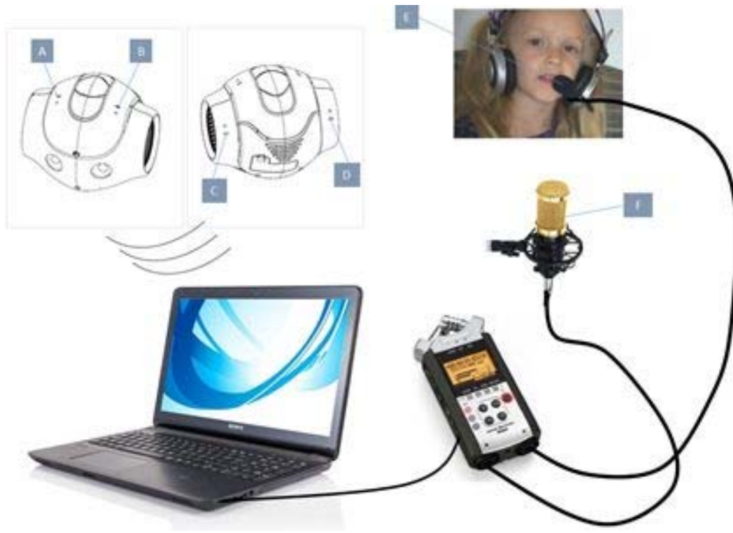
Figure 1 - Data Collection framework: A,B,C,D - 4 microphones of Nao (the robot used in the ALIZ-E project); E - 1 close-talk microphone; F - 1 panoramic microphone.
